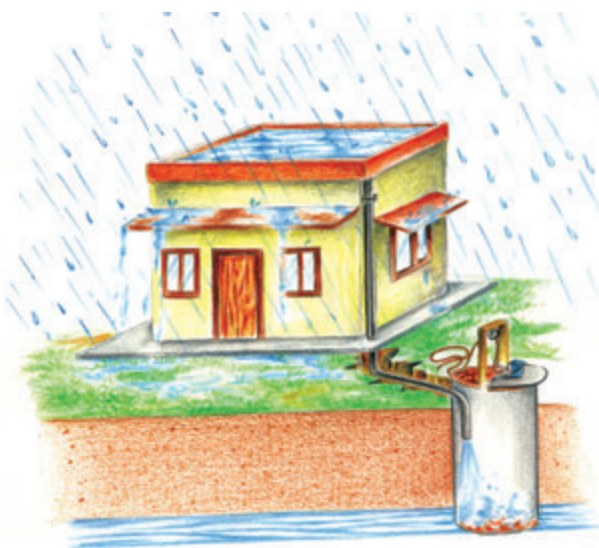
(b) Recharge through Abandoned Dugwell
