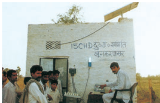
Fig. 5.11: Solar operated electronic milk testing equipment
