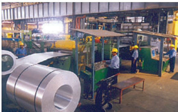
Fig. 6.6: Strip casting mill at smelter of NALCO
