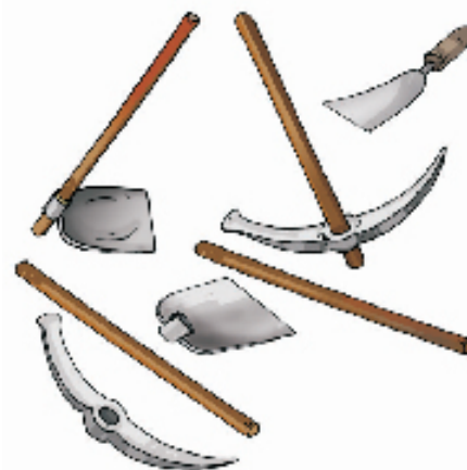
Fig 6.6 Tools are often heated before fixing wooden handles
