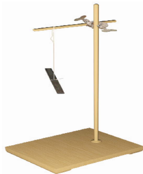
Fig 13.9 A freely suspended bar magnet always comes to rest in the same direction
