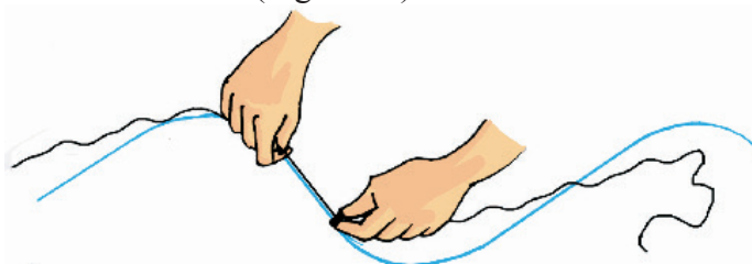
Fig 10.10 Measuring the length of a curved line with a thread
