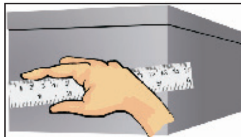
Fig 10.8 (a) incorrect and (b) correct method of placing the scale with broken edge
